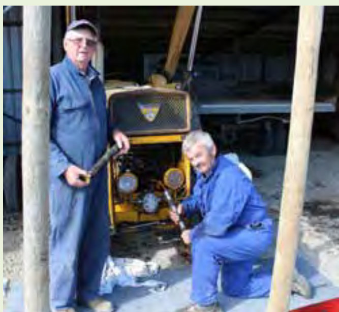
Graeme and Brian carrying out some repairs on the Massey Ferguson steering. Some new bushes are being fitted to the steering shaft.
